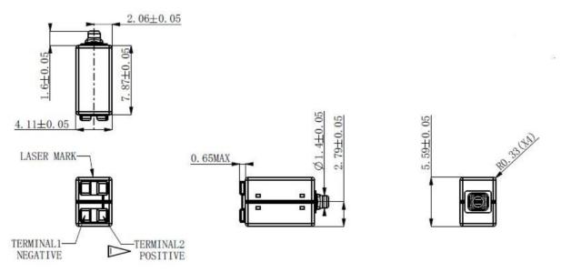
\*A positive voltage applied to the negative terminal (-) will result in an increase in pressure at the sound outlet.
