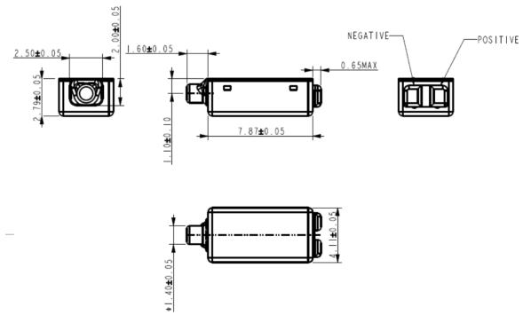
\*A positive voltage applied to the negative terminal (-) will result in an increase in pressure at the sound outlet.
