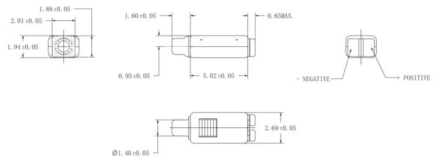
\*A positive voltage applied to the negative terminal (-) will result in an increase in pressure at the sound outlet.
