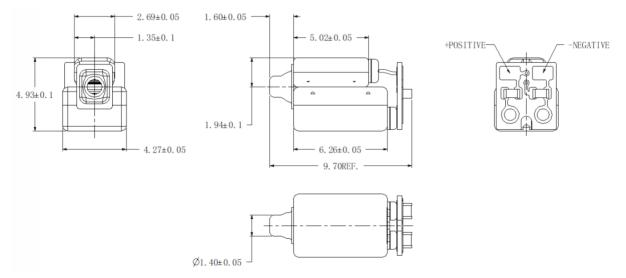
\*A positive voltage applied to the negative terminal (-) will result in an increase in pressure at the sound outlet.
