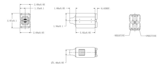
\*A positive voltage applied to the negative terminal (-) will result in an increase in pressure at the sound outlet.
