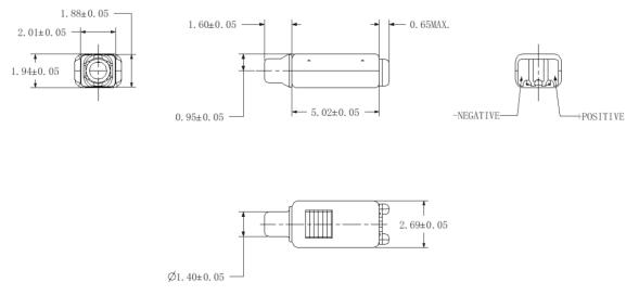
\*A positive voltage applied to the negative terminal (-) will result in an increase in pressure at the sound outlet.
