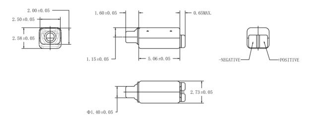
\*A positive voltage applied to the negative terminal (-) will result in an increase in pressure at the sound outlet.
